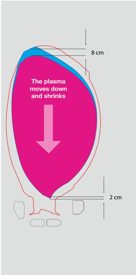
*Moderating Edge Localised Modes (ELMs): An additional voltage pulse to the vertical stability coils momentarily move the plasma down a few centimeters and shrinks it, triggering an ELM each time.*
