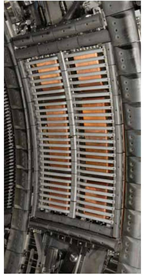
*The ITER-Like Antenna fully mounted in JET. Hidden behind the rods, but clearly visible, are the copper 'straps' that radiate the power into the plasma.*
