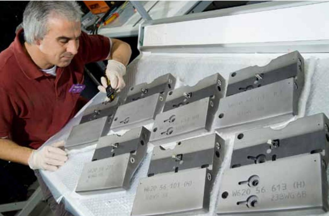
*The shutdown commenced on 26 October. Here, Rob Fenn is in the JET Clean Room, inserting the fixing bolts for the individually numbered tungsten tiles.*
