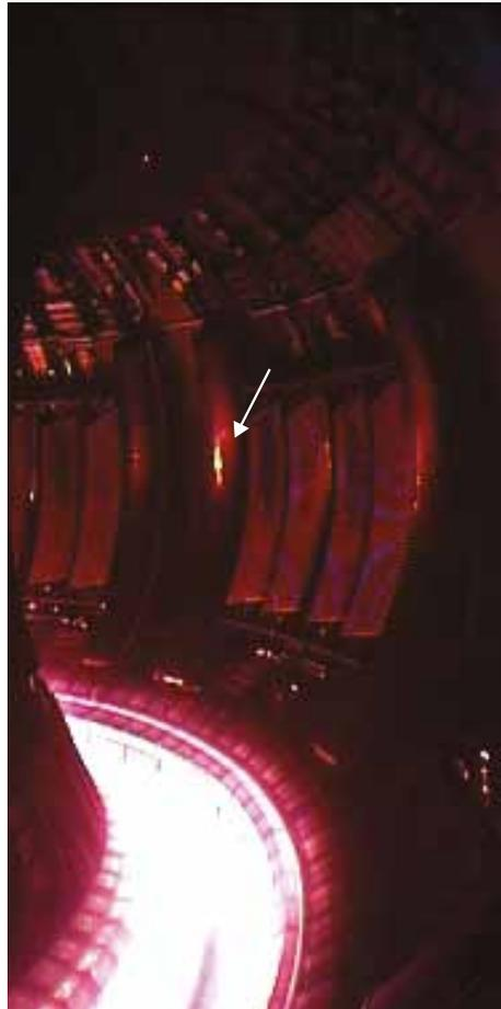
*Picture taken with visible light camera shows Toroidal Field ripple induced losses (indicated by the arrow) on the poloidal limiter for a plasma with one per cent ripple. The experimental results are consistent with the calculations done beforehand.*
