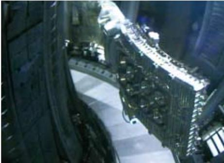
The boom transports the antenna within the vessel to its final location.
