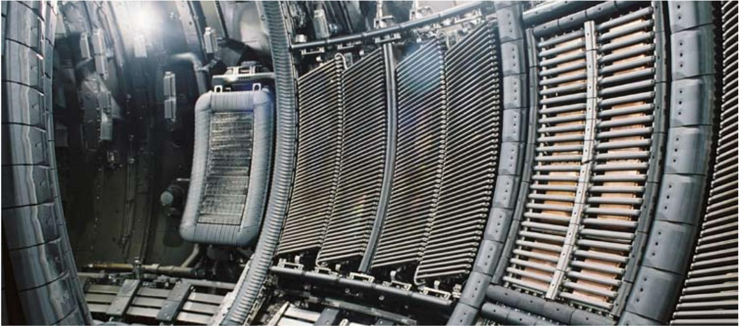
A look inside the vessel: The three rectangular elements are antennas for heating systems available at JET; (from left) the Lower Hybrid, the ICRH and the ITER-like ICRH.
