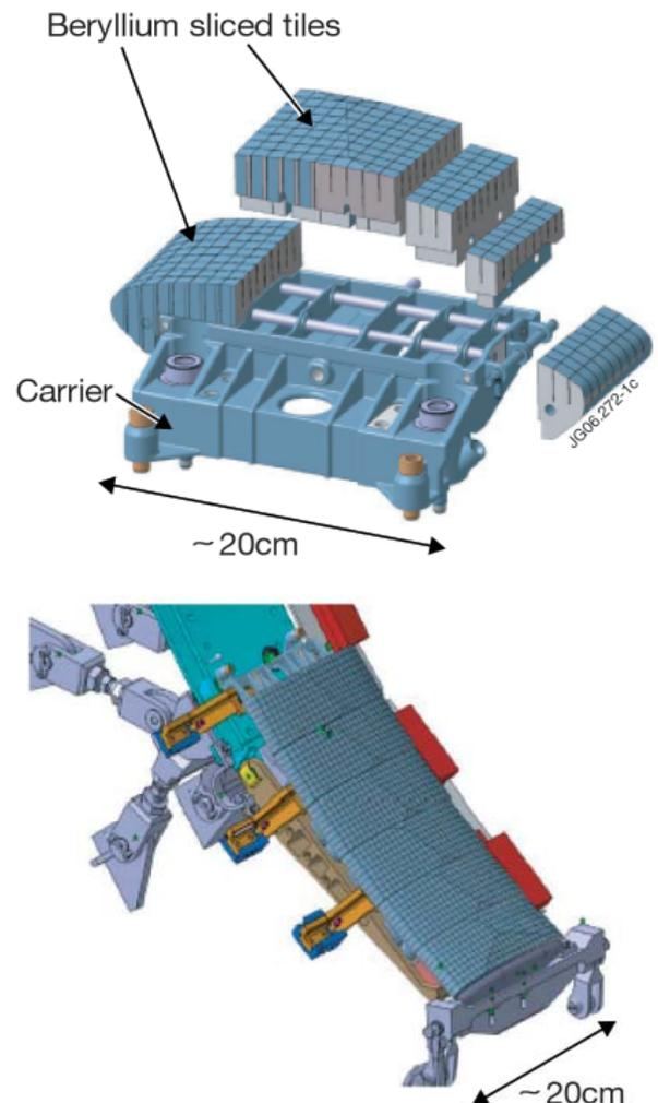
Figure 1: Example of tile design for the JET main wall structure (here a poloidal limiter)
