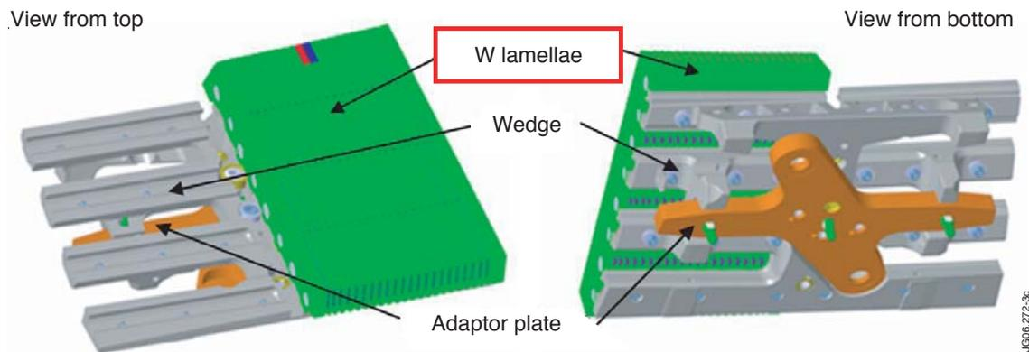
Figure 3: Example of the design of a bulk tungsten tile for the heavily power-loaded areas of the future JET tungsten divertor.
