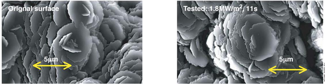
Figure 2: Scanning electron microscope image of a beryllium coated tile before and after the high heat flux test. The comparison shows that the coating survived the test without loss of quality.
