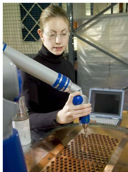
Accelerator grid undergoing alignment checks during PINI assembly. New grids with enlarged beam extraction apertures will be manufactured for the Neutral Beam Enhancement Project.
