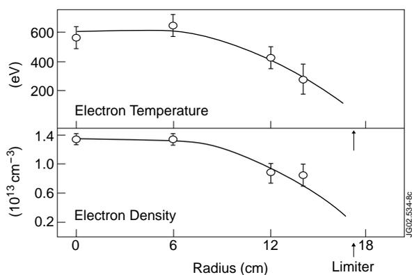
*Radial variation of electron temperature and density. The lines shown are drawn through the experimental points. ( $I_s = 60\text{kA}$ ,  $H_s = 17\text{kOe}$ ,  $t = 25\text{ms}$ )*
