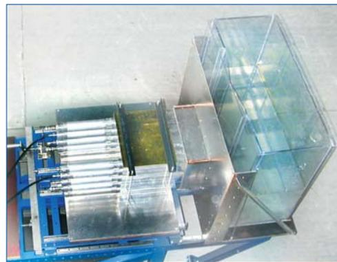
Fig. 3. Mock-up of the antenna array, mounted in front of a water tank on a sliding table for controlling the distance between the array and the water load. The 8 outputs of the 4-ports junctions, where the measurement of the S matrix is done, are seen on the left side of the picture.
