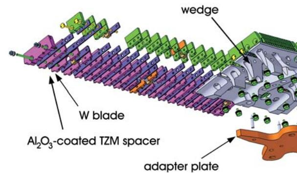
The lamellae concept consists of stacks of tungsten and insulating spacers, held together by tie rods and being mounted onto a support structure. Differences in thermal expansion of the materials involved and mechanical pre-tension – being required to avoid detachment in case of electromagnetic loads due to disruptions
