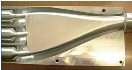
Fig. 2. Photo of the inner part of one antenna triplet, fed by a 4-ports junction. The scale is 1/5.
