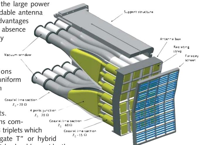
Fig 1. Design of an ICRH antenna plug for ITER.
