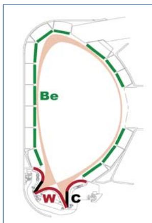
*Reference design for ITER first wall; backup/second stage design has an all-tungsten divertor*
