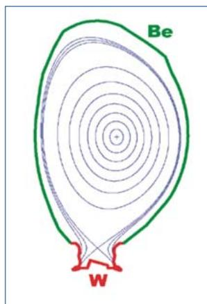
*Reference design for wall change on JET - matches ITER backup/second stage design.*
