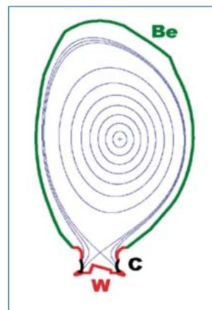
*Alternative design for wall change on JET - matches ITER reference design*
