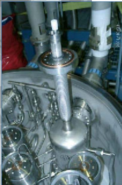
Installation of a new cryopanel prototype at JET (C. Day, EURATOM-Association-FZK)
