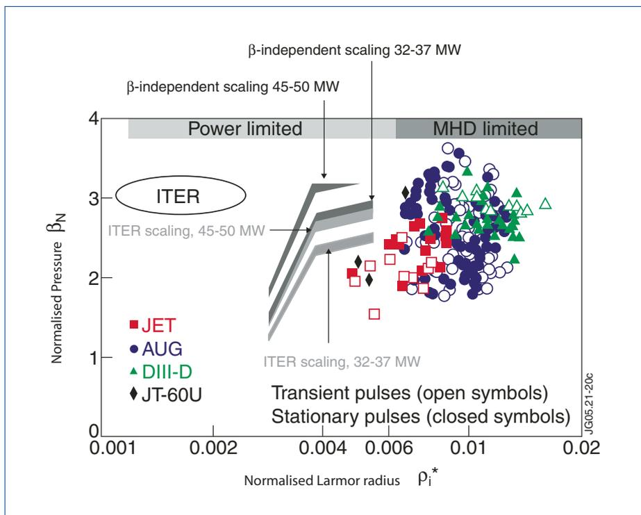
*Access to the Improved H-mode at low rho-star and high beta is limited by available power on JET. The NB power upgrade will allow studies of this scenario much closer to the ITER operating point, than is currently possible.*
