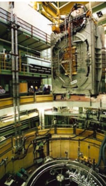
The Euratom LCT coil, providing the background field for the test of TFMC, was also tested alone: first at a winding temperature of 4.5 K to a maximum current of 11.3 kA, and later at a winding temperature of less than 3.1 K to a maximum current of 16 kA. Finally the coil assembly was energized to the rated values of 70 kA in TFMC and 16 kA in LCT. This corresponds to 8.78 T maximum field at the conductor of the TFMC and 282 MJ of stored energy in both coils.
