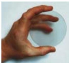
*A number of years of co-development with industry has led to a solution using an ideal material: diamond. It has very low absorption, high strength and good thermal conductivity. The example here is 80 mm diameter and 1.5 mm thick.*
