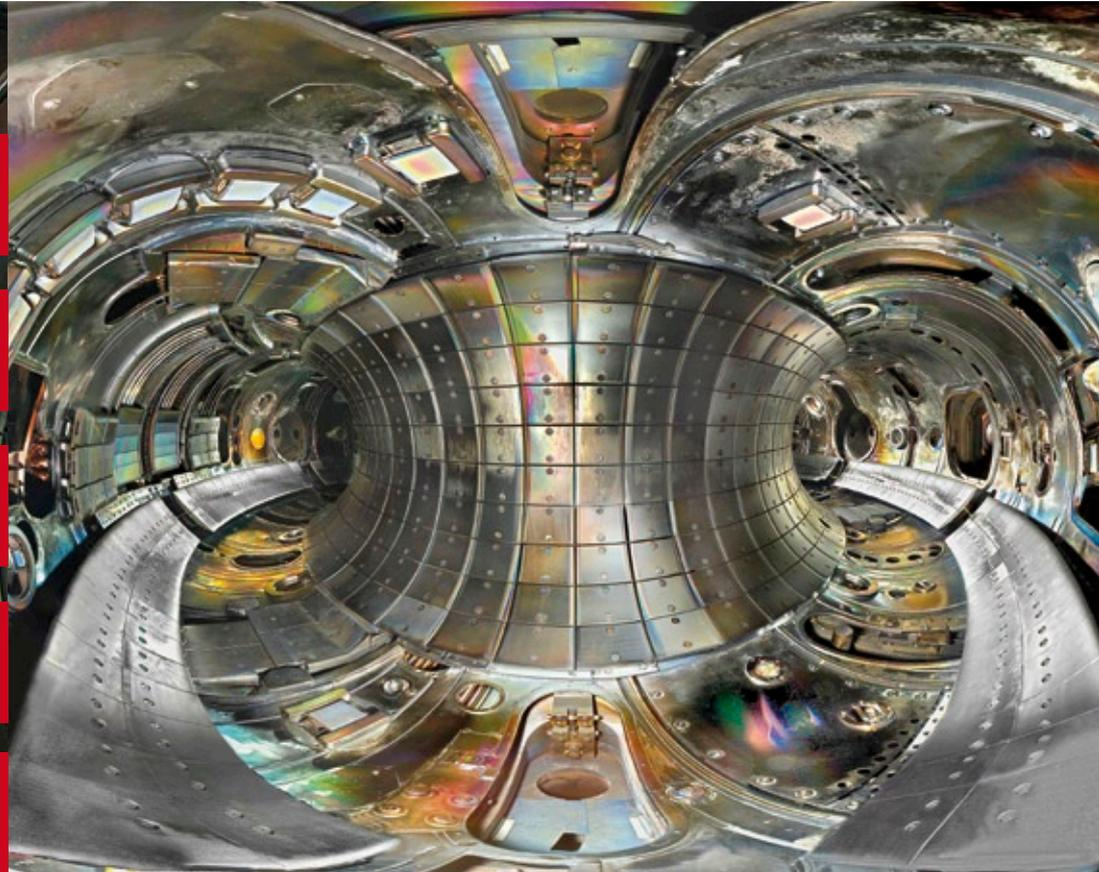
Panoramic view into the burn chamber of the TEXTOR tokamak at Forschungszentrum Jülich. The machine is specialised for material and Plasma Wall Interaction research (see the PWI article in this issue). To investigate how particle and energy transport in the plasma edge can be influenced by resonant magnetic perturbations, TEXTOR is equipped with the unique Dynamic Ergodic Divertor. (Photo: Harry Reimer, Forschungszentrum Jülich, April 2009)
