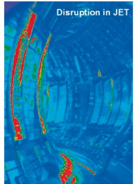
Heat flux patterns on the vessel walls during a disruption in JET. The red areas correspond to the plasma facing components heated by the disruption. The divertor is at the bottom of the vessel. (Photo: EFDA JET)
