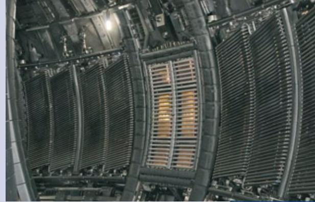
The ITER-like Antenna ILA (installed in 2007, 7.2MW, 0.9m<sup>2</sup>) between two A2 antennas (1996, up to 4MW, 2.2m<sup>2</sup>) inside JET. The copper coloured areas behind the bars of the Faraday Screen are the straps of the ILA. (Photo: EFDA JET)
