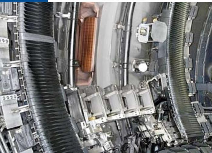
Fig. 2 Toroidal Alfvén Eigenmode antenna array installed in JET
