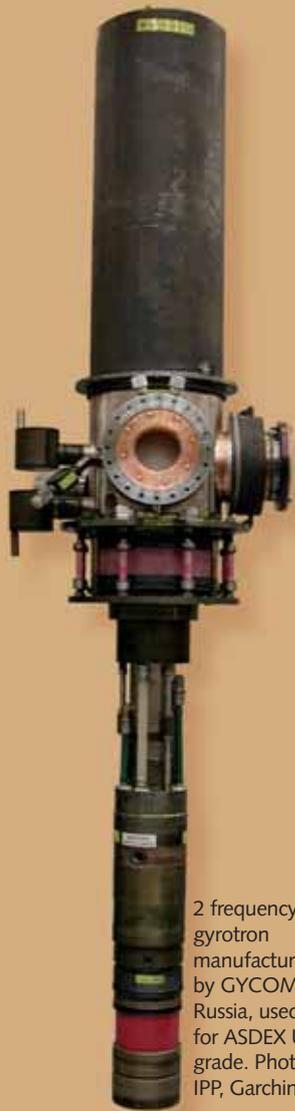
2 frequency gyrotron manufactured by GYCOM, Russia, used for ASDEX Upgrade. Photo: IPP, Garching
