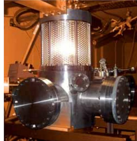
A microwave plasma is activating the gas mixture to deposit a diamond coating on to a substrate below.
